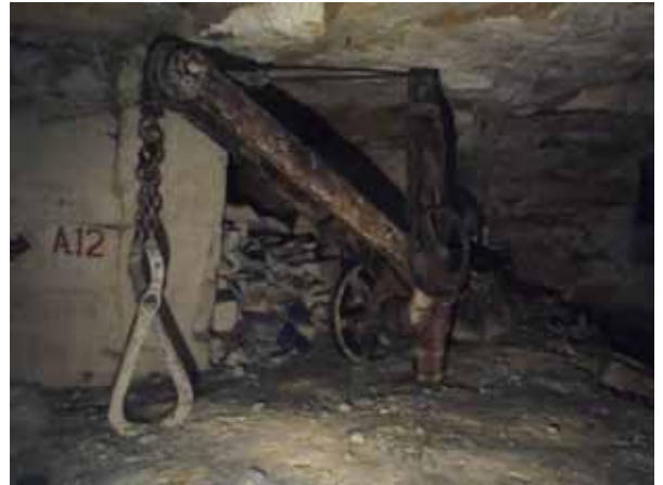
Figure 14.10 An old crane survives underground at the freestone mines at Corsham in Wilts. © Richard Shaw
