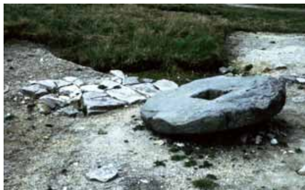
Figure 7.11 A crushing circle excavated at High Rake Mine in Derbyshire. The crushing stone or edge runner is in the foreground and vestiges of the track are behind. © Dave Williams
