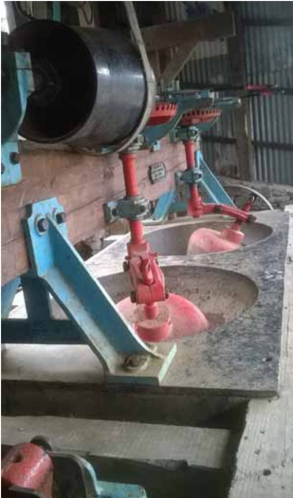
Figure 10.2 No Berdan gold amalgamation pans survive in England but two Britten pans, a later development on the same principle, have been preserved, albeit not in situ, at Coed-y-Brenin, Merionethshire. © Peter Cloughton
