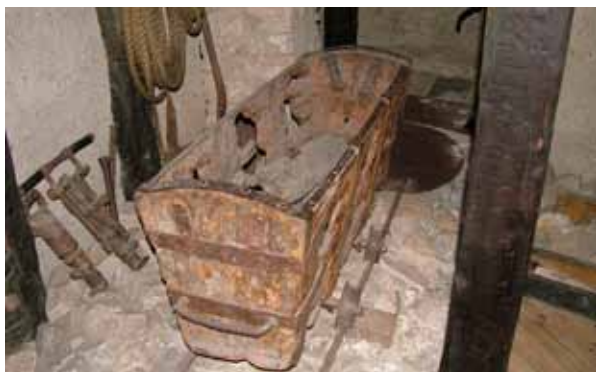
Figure 7.10 An early wooden tram waggon which ran on metal rails, now on display at the Peak District Lead Mining Museum. Phil Newman
