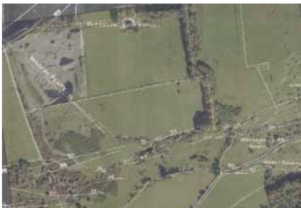
Figure 13. 4 An overlay of part of a scanned 1840s map of the mines on Longstone Edge, Derbyshire onto publicly-available satellite imagery from Google Earth™, allowing identification of vein and shaft locations obscured by modern fluorspar extraction. Images © of the Derbyshire Record Office and Google, overlaid by Adam Russell.
