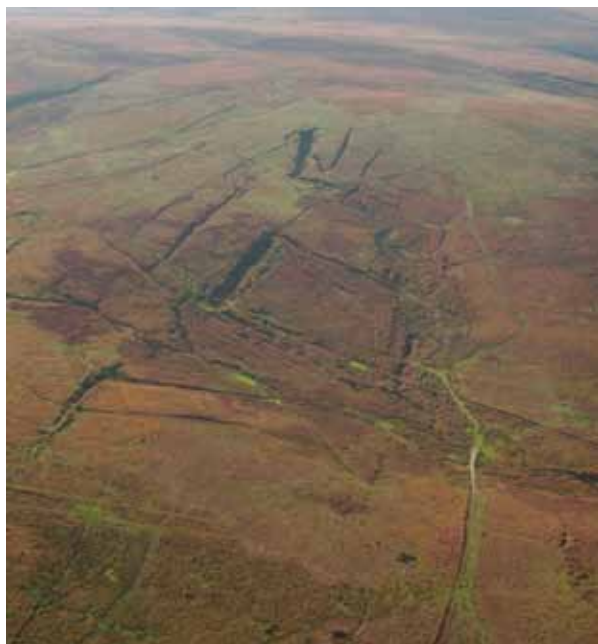
Figure 8.5 Openworks, where shallow tin lodes were worked using an open-cast method at Ringleshutts, Devon. Damian Grady, © Historic England
