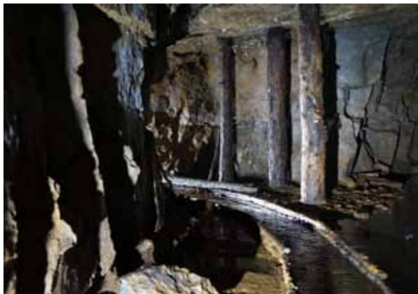
Figure 14.9 Harnisha Burn Lead and Fluorspar Mine, Frosterley, Durham. Nineteenth century lead mine horse level reopened as a fluorspar mine around 1970-5. Timber roof supports and steel rails are from the 1970s reopening. © James Heaton
