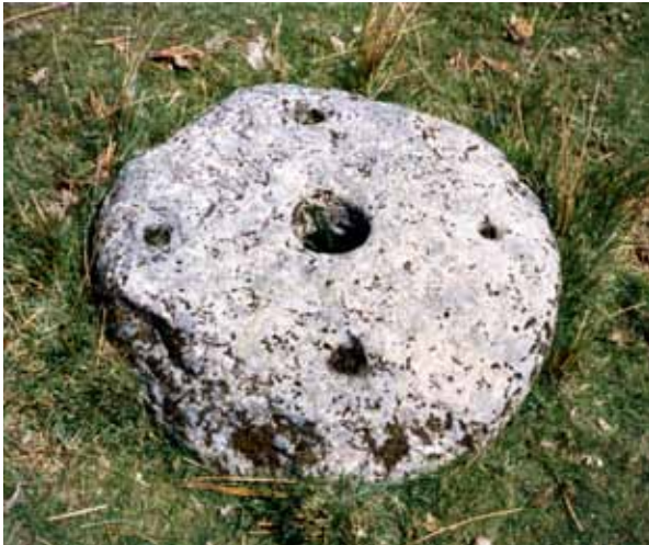
Figure 8.2 The upper stone of a crazing mill at Gobbett in Devon. This rare survivor formed one half of a rotary mill used for dressing tin. Untypically, the lower stone also survives at this site, as does evidence for smelting in the form of a mouldstone. © Phil Newman
