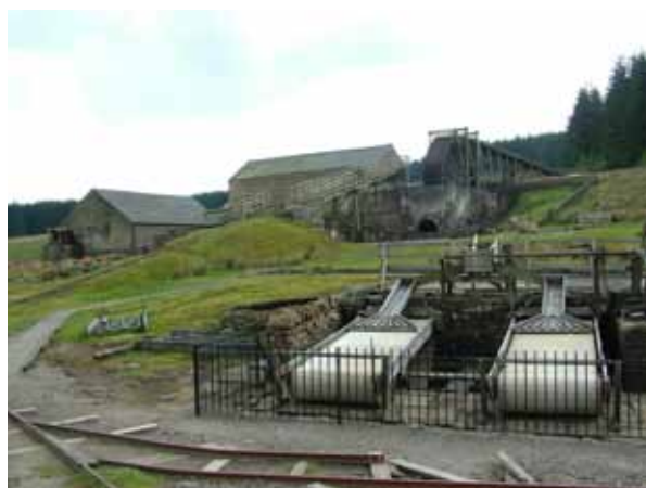
Figure 7.12 Killhope Lead Mine in Weardale Co. Durham is now run as a lead mining museum. The large waterwheel once powered a crushing mill. In the foreground are restored Brunton frames. © Phil Newman
