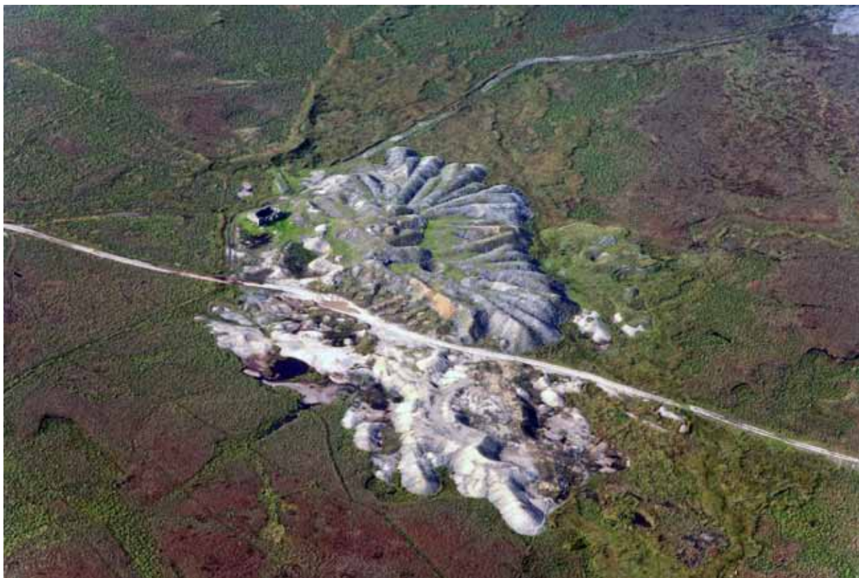
Figure 7.3 Aerial view of Old Moss Mine on Grassington Moor in the Yorkshire Dales showing finger dumps of waste. © NMRS
